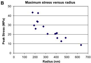
**Fig. 4.** (A) Plot of modulus vs radius. The modulus decreases with increasing radius. (B) Plot of maximum stress vs radius. The maximum stress decreases with increasing fiber radius.
