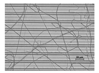
**Fig. 2.** Optical microscope image of the electrospun collagen type I sample. The ridges are visible as darker gray horizontal stripes  $8 \, \mu m$  wide and are spaced by lighter gray  $12 - \mu m$  grooves. The electrospun fibers are randomly oriented on the surface. Fibers aligned perpendicular to the ridges are selected for manipulation.
