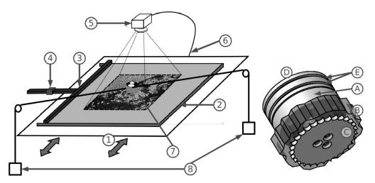
Fig. 1. Left: Original experimental setup and additional rheometer device. Right: The rheometer-wheel (see text for details).
